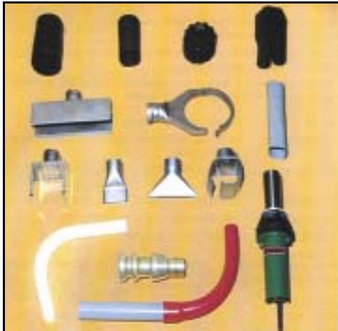
Tools currently available for shrinking and bending of thermoplastics
